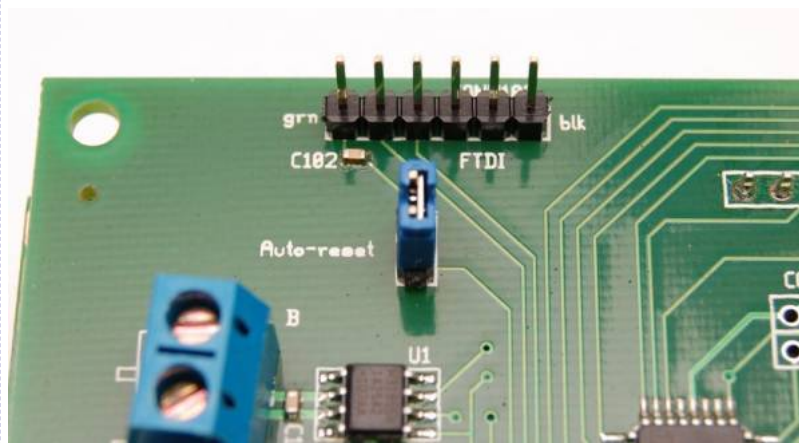
Auto reset jumper, disable auto reset by disconnecting the jumper
